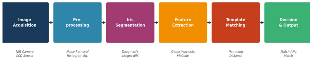
Fig. 1 Block diagram of the proposed iris recognition pipeline. Arrows denote information flow between processing stages.
