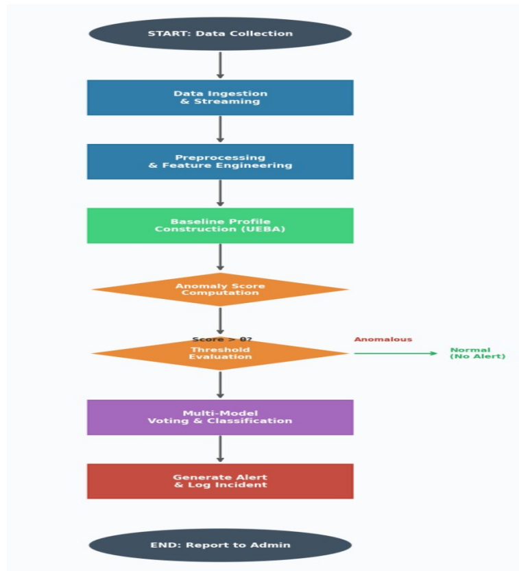
Fig. 2 Detection and classification flow diagram illustrating the decision pipeline from data ingestion to alert generation
