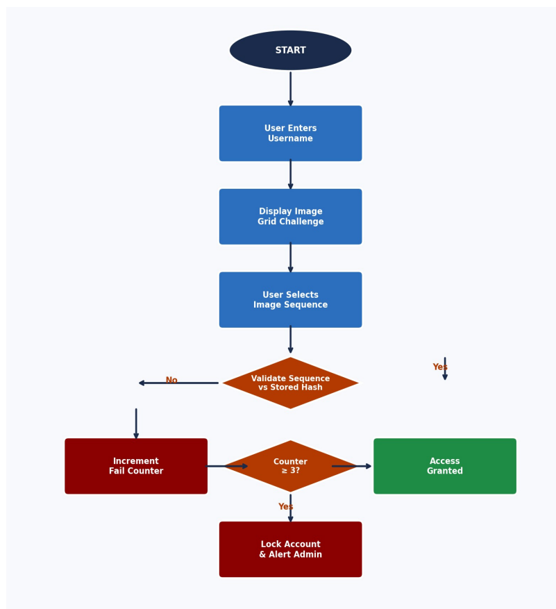
Fig. 2 Knowledge-Based Authentication Process Flow for the Proposed GBPA System
